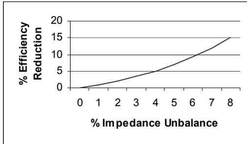
**Figure 1:** Efficiency Reduction Due to Impedance Unbalance
