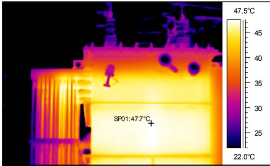
**Figure 5a.** LN Regulator No. 1 winding section before filling
