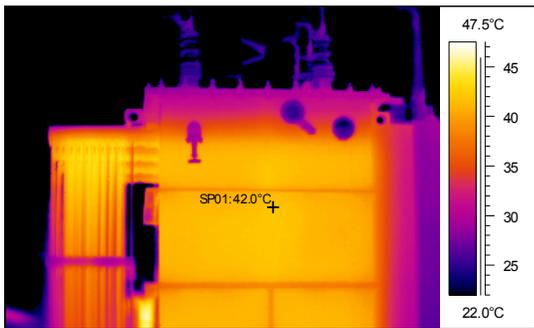
**Figure 5c.** LN Regulator No. 2 winding section before filling
