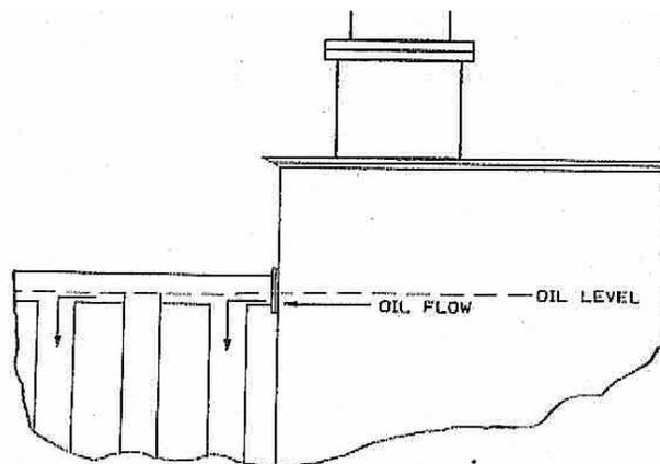
**Figure 3. The oil level must be above the upper flow pipe for proper cooling.**
