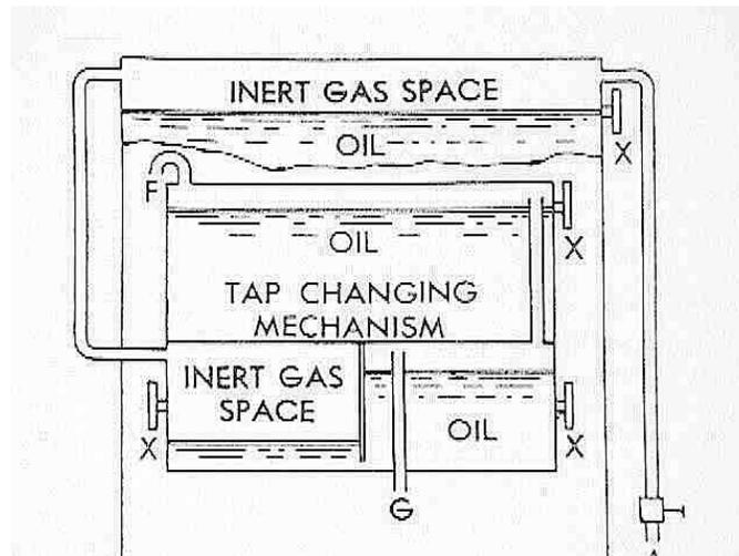
**Figure 1. Configuration of the 3 chambers of a typical regulator**
