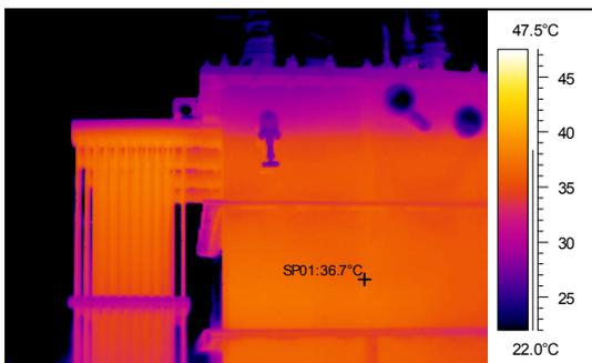
**Figure 5e.** LN Regulator No. 3 winding section before filling
