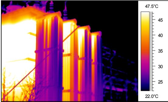
Figure 4a. LN Regulator No. 1 radiators before filling
