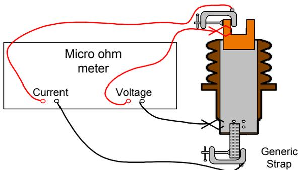
Micro-ohm testing of a Bushing which checks the conductor integrity
