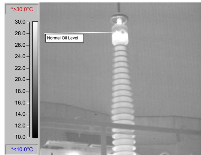
Oil level can be detected on transformer bushings because the windings produces a heat source that heats the oil in the main tank and the bushings. The bushings have an oil expansion chamber at the top. Since the oil has a higher thermal mass than the void, the expansion chamber temperature profile shows the oil level. This is then checked to see if this matches the gauge or site glass.
