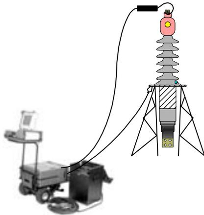
Powerfactor testing of a Bushing which checks the insulation integrity
