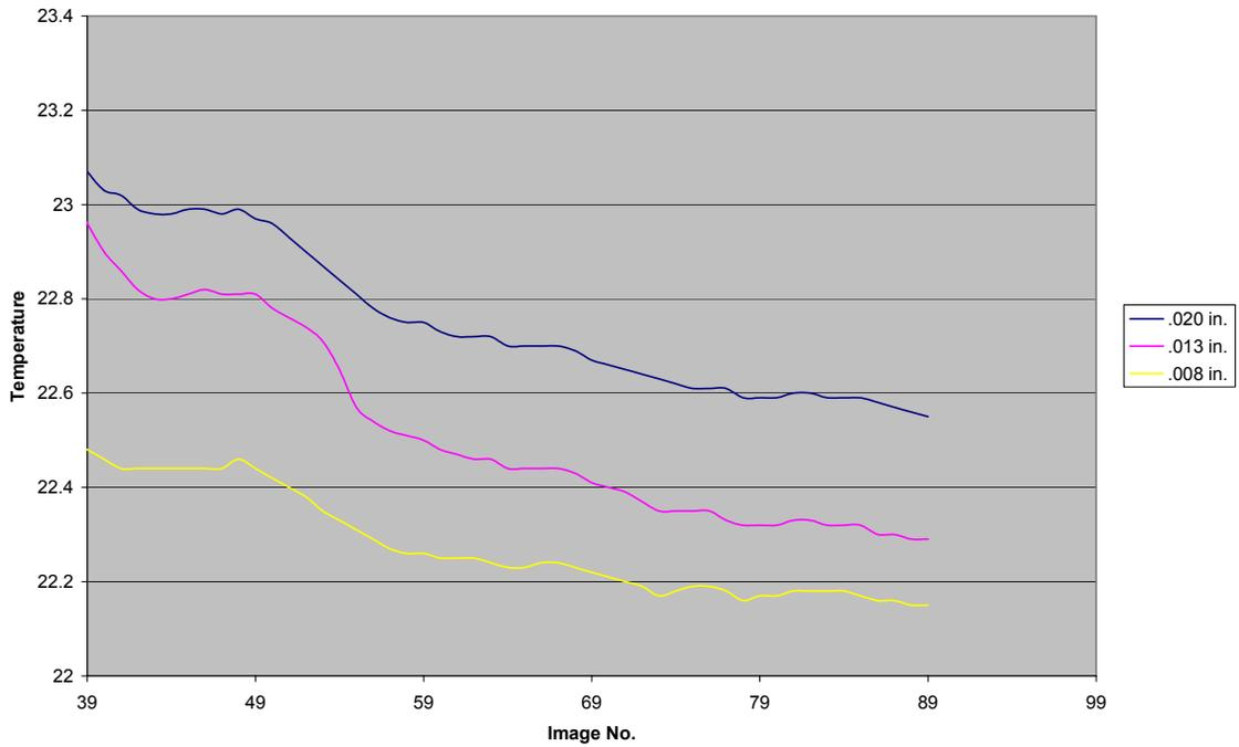
Figure 2. Thermographic Decay Curve Quantum Well IR Test
