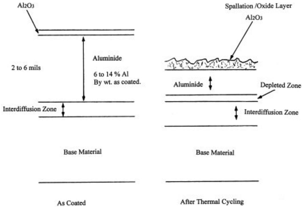
Typical NiCrAlY overlay coating – As coated vs. after thermal cycled.
