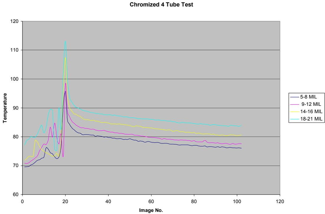
Figure 5. Chromized Tube IR Test 5-8,9-12,14-16,and 18-21 mil thickness
