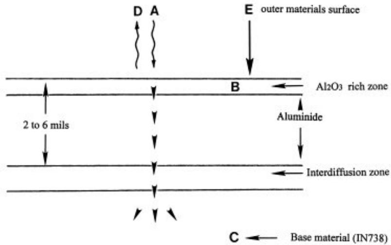
Basic heat flow conditions during thermographic test sequence.
